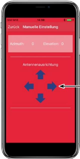
10. In the „Manual Adjustment“ menu, rotate the antenna with the left and right arrows for azimuth, or rotate the antenna with the up and down arrows for elevation.
