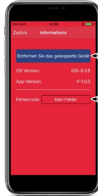
11. If you want to separate the app with the control device, press this field. You can then pair with another or new control device.
