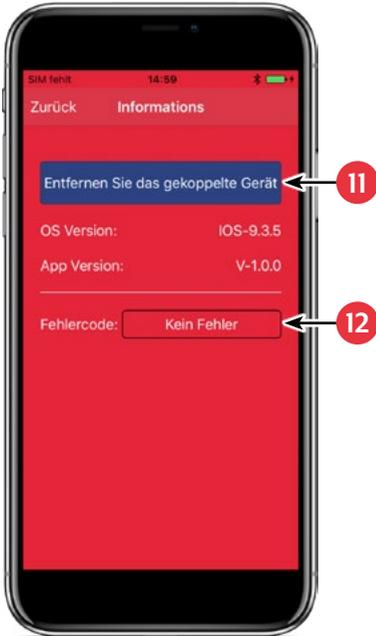
11. If you want to separate the app with the control device, press this field. You can then pair with another or new control device.
