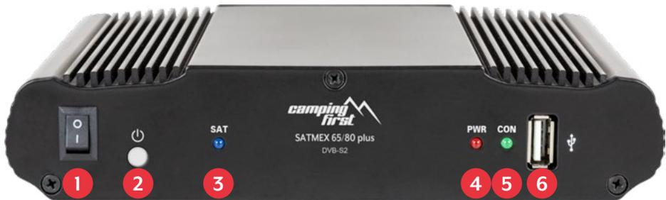
1. I/O: Main switch for power supply.
