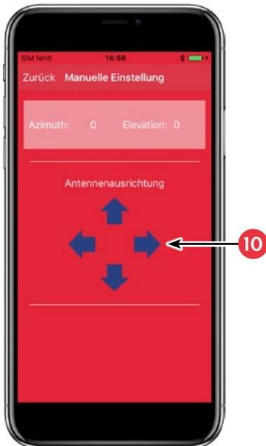
10. In the „Manual Adjustment“ menu, rotate the antenna with the left and right arrows for azimuth, or rotate the antenna with the up and down arrows for elevation.
